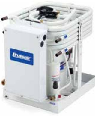
The new RM model remote modulating condensing units are the next generation of direct-expansion, cooling only air conditioning units designed to run multiple cooling units (evaporators) with up to five independent zones. Models are available in capacities of 24, 30 and 42,000 BTU/Hr. Total cooling unit capacity should be within 15% of the condensing unit capacity.
