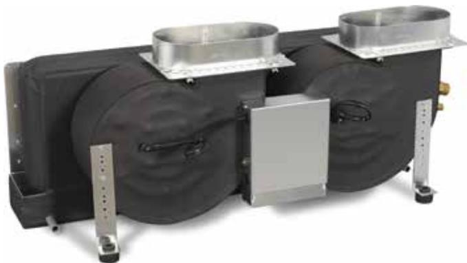
Cruisair's EBLE low profile, dual-blower series of ductable cooling/heating units are available in a wide range of capacities and configurations. Available in capacities from 12K to 36K BTU/hr., EBLE units are designed for installations where there is limited vertical space, such as beneath a seat or bunk, or in overhead spaces.
