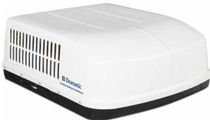
The DuraSea Rooftop is a 15,000 BTU/hr air conditioner\* built to endure harsh marine environments. Ideal for patrol boats, house boats, and other vessels, it is designed to be installed on a flat deck or rooftop and cool the area directly below. It is air cooled and requires no plumbing or ducting.
