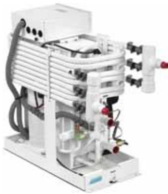
Marine Air's MCG chilled water series is available in capacities ranging from 24,000 (2 ton) to 180,000 (15 ton) BTU/hr. Featuring a compact base design, MCG modules can be staged to provide a larger system, which is easily retrofitted and serviced in the field. Up to six 15-ton stages can be configured for a system total of 1,080,000 BTU/hr, or 90 tons.
