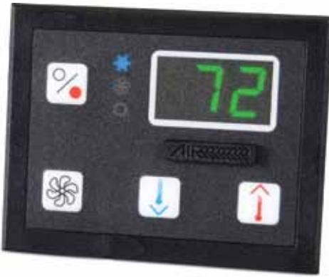
The Passport I/O Environmental Control Unit is a microprocessor based controller, designed for the precise control and monitoring of direct expansion and chilled water boat air conditioning systems from Marine Air. The control is dual voltage, operating at both 115 and 230 Volts, 50/60 Hz. The display is available in both black and white. In chilled water air handlers, the control is referred to as AH-Passport I/O.
