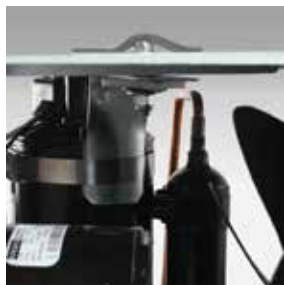
Compressor is bracketed at top as well as bottom to minimize vibration and movement while under way.
