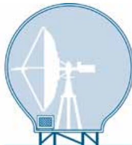
Interior dome self-contained (exhaust kit is available for low pedestal applications to correct condenser air short cycling)
