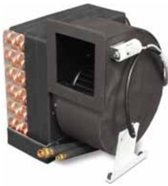
Compact EBE split evaporators for boats are draw-through, ductable cooling units with reverse-cycle heating. Featuring a rotatable, high-efficiency permanent split capacitor (PSC) blower in which the motor is concealed, EBE series evaporators are available in capacities from 6K to 36K BTU/hr. EBHE units have electric heat.
